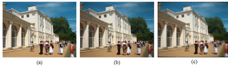
Fig. 9. Comparison of image simulations before and after optimizing the SLR system. (a) The source image for the simulation (b) The simulated image after optimization (c) The simulated image before optimization but after modifying parameters from the Double Gauss sample file.
